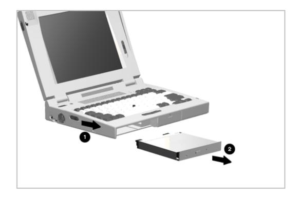
Figure 5-13. Removing a Device from the MultiBay
